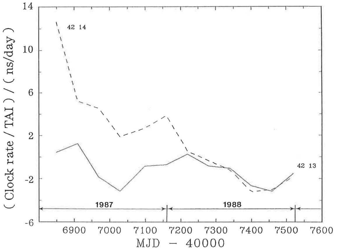
Fig. 2: Frequencies relative to TAI of the two H-masers APL 13 and APL 14 for a 20-month period. These H-masers were taken out of operation at the beginning of 1989 and reintroduced in TAI computation in 1990.
