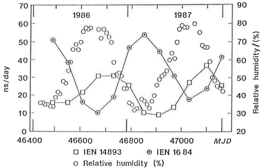
Fig. 6: Variation with time of the frequencies relative to TAI of IEN 14 893 and IEN 16 84 and relative humidity in the room where they are kept.
