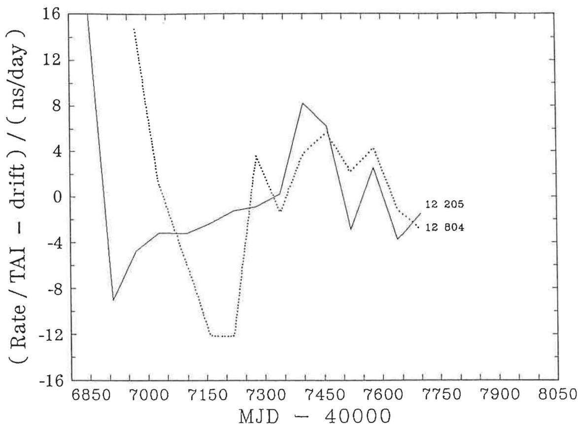
Fig. 10: Variation with time of the frequencies relative to TAI of ORB commercial caesium clocks 12 804 and 12 205 after drifts removing (respectively:  $-0,057\text{ns/day}^2$  and  $-0,045\text{ns/day}^2$ ).
