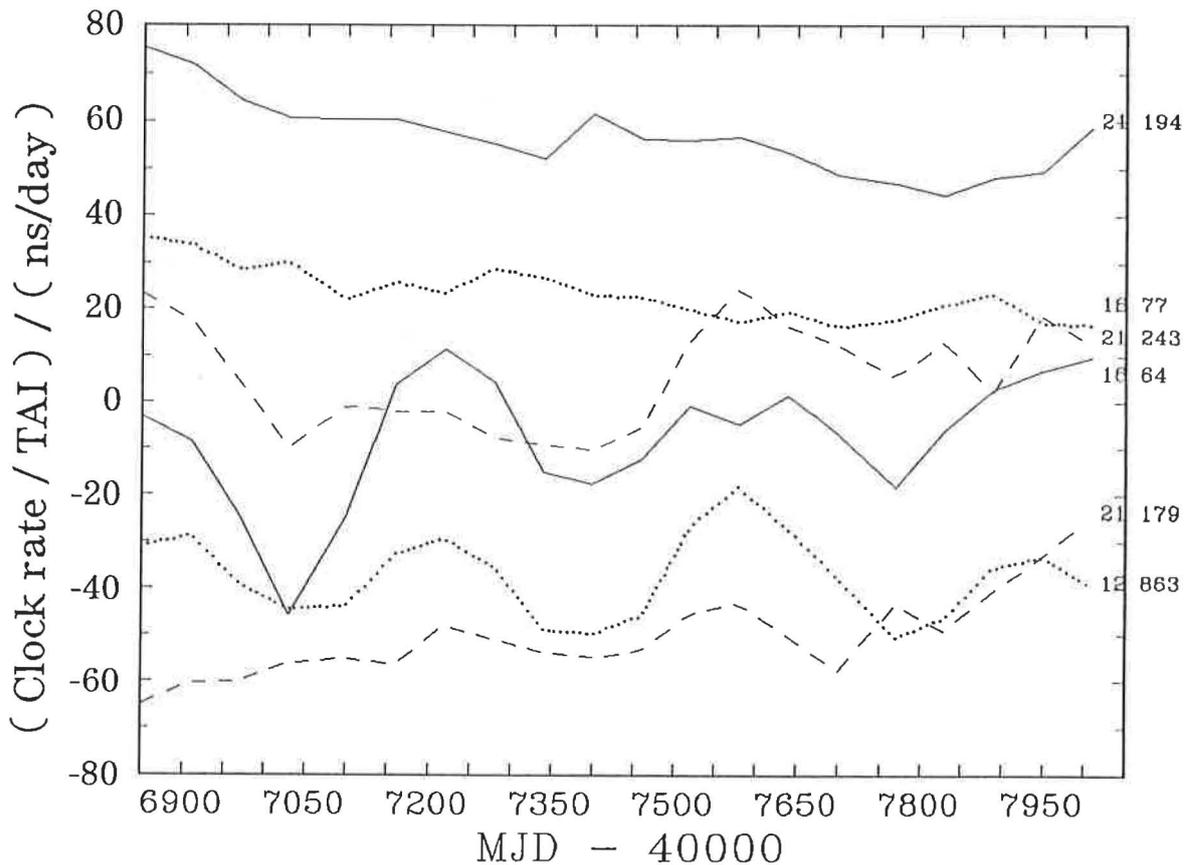
Fig.13: Frequencies relative to TAI of six CH clocks (all of them are of commercial type). Clocks kept by the same swiss laboratory are represented by the same line type.
