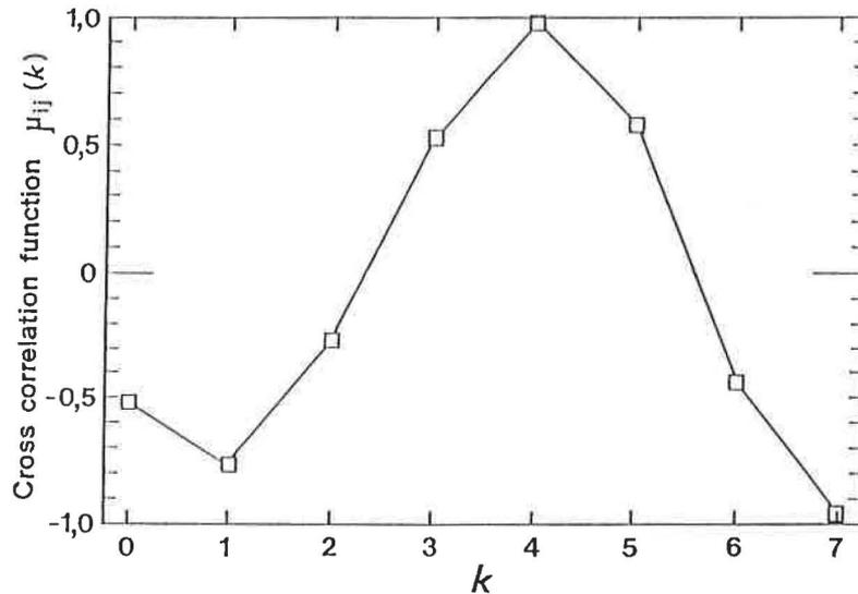
Fig. 7: Cross-correlation function  $\mu_{ij}(k)$  (as defined in Section I) versus lag  $k$ , for the two clocks IEN 14 893 and IEN 16 84.
