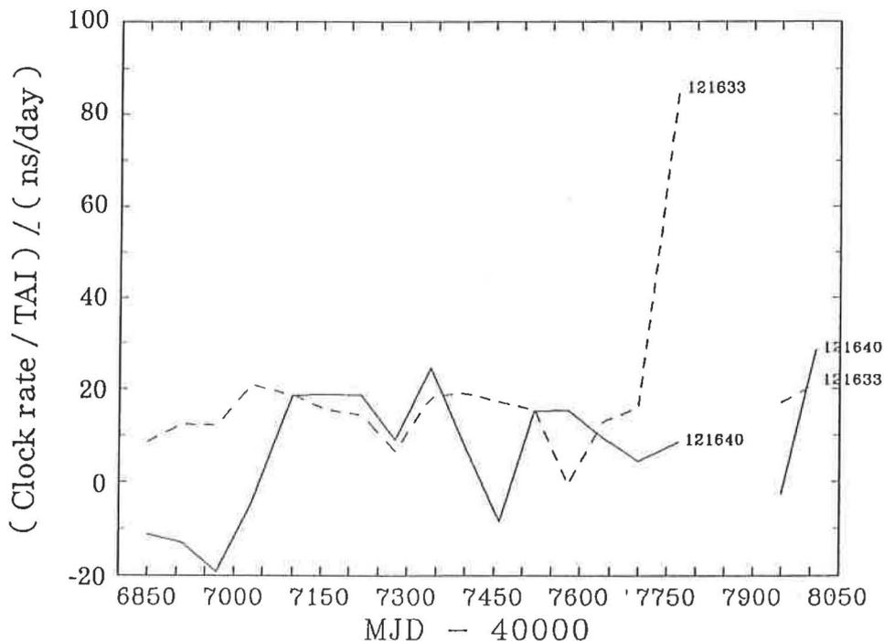
Fig. 21: Frequencies relative to TAI of NIM clocks, general overview (Clock 121615 is not shown).
