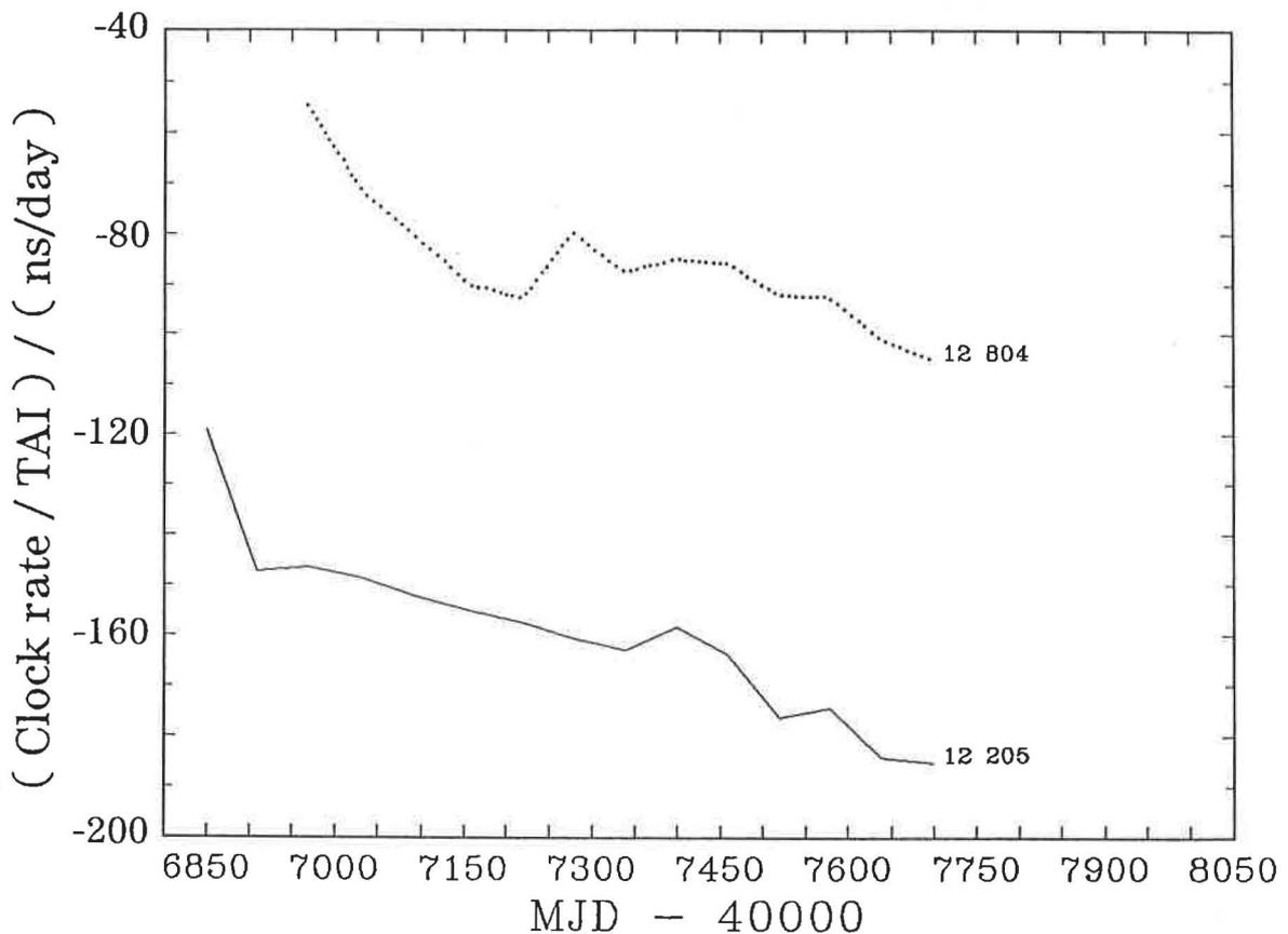
Fig. 9: Variation with time of the frequencies relative to TAI of ORB commercial caesium clocks 12 804 and 12 205. Their performance after MJD 47699 is ignored because both of them had a frequency step.
