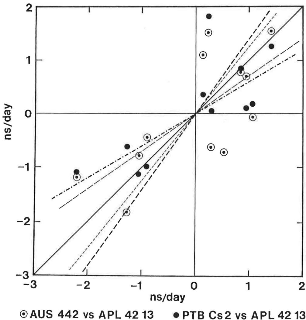
Fig. 4: Frequencies relative to TAI of APL H-maser 44 2 and PTB primary standard CS2 versus the frequency relative to TAI of APL H-maser 42 13 (the frequency values are reduced to their averages)
