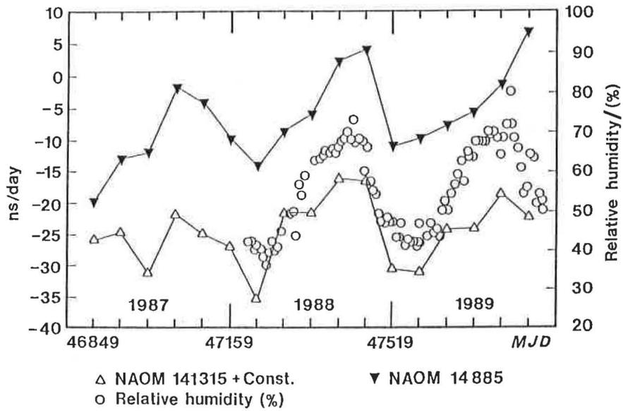
Fig. 5: Frequencies relative to TAI of NAOM 14 885 and NAOM 141315 and relative humidity in the room where they are kept.
