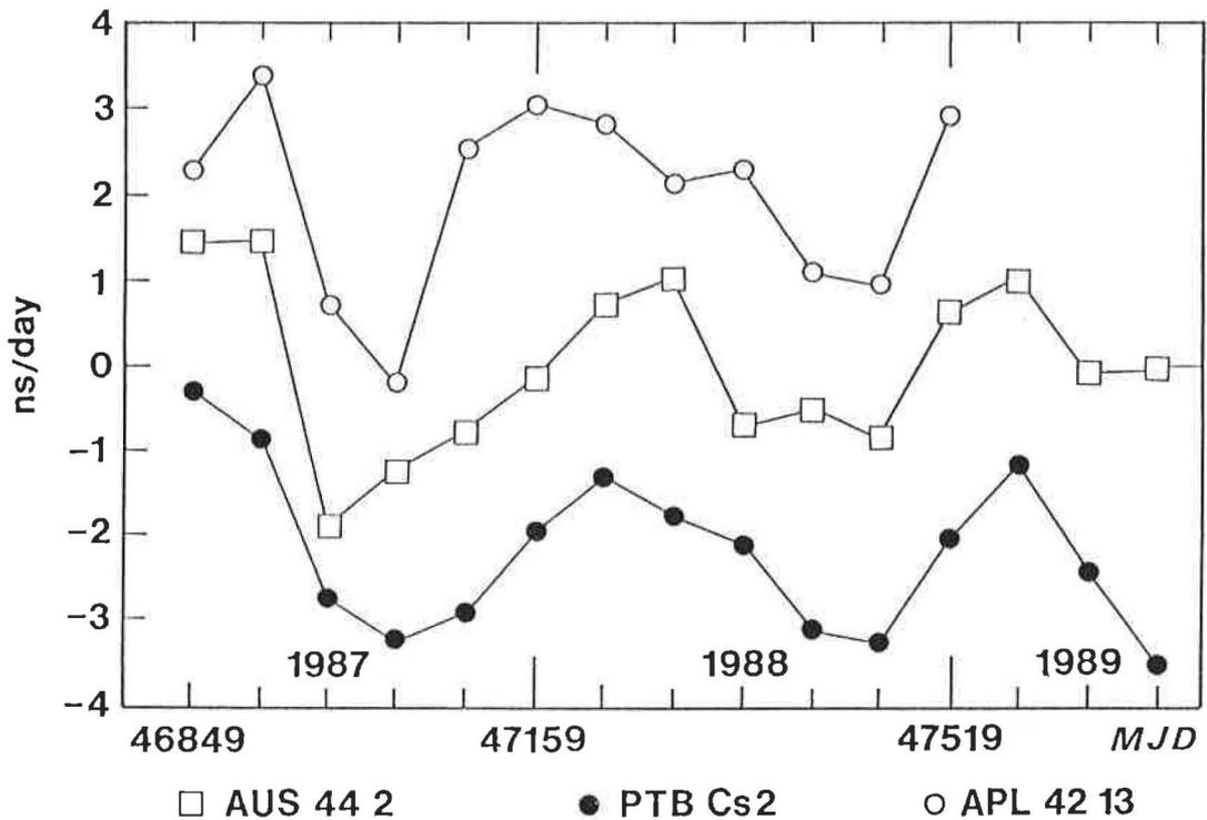
Fig. 3: Frequencies relative to TAI of APL H-maser 42 13, AUS H-maser 44 2 and PTB primary standard CS2. The H-maser values are globally shifted and the drifts removed.
