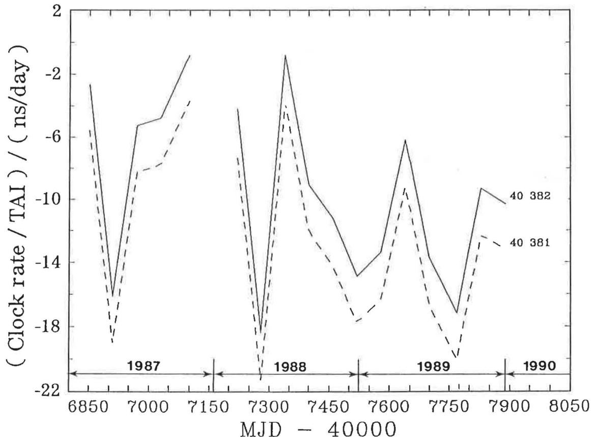
Fig. 8: Variation with time of the frequencies relative to TAI of SU H-masers 381 and 382 (the frequency values are shifted by 3ns/day for SU 382).
